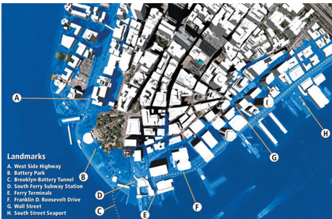
FIGURE 6-10 The challenge of rising sea level and the expansion of the one percent annual chance floodplain to New York City. The light blue area represents a 2012 depiction of the one percent annual chance floodplain of Lower Manhattan, New York City. With sea-level rise, a far larger area would be flooded in the event of a one percent annual chance flood event. (Note that flooding during Hurricane Sandy (2012) exceeded the one percent annual chance flood.) With sea-level rise, the one percent annual chance flood will inundate a larger area of New York City (not pictured here).
